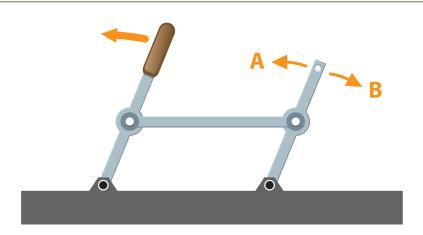
As the handle is pulled, in which direction will the end of the bar move?
