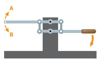
In which direction will the arm swing when the handle is moved as shown?
